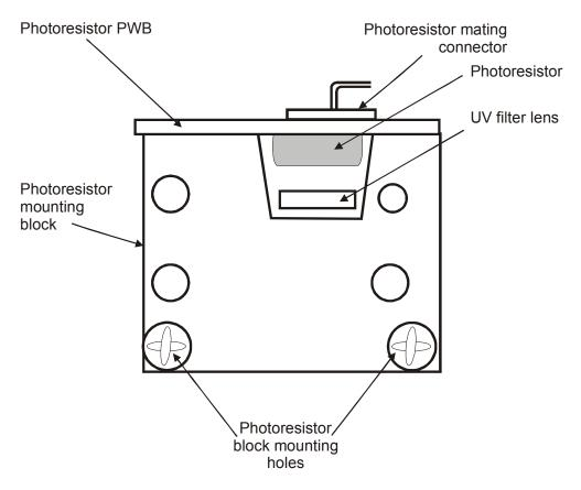
Figure 41. Photoresistor Assembly for Direct View (I300M)
